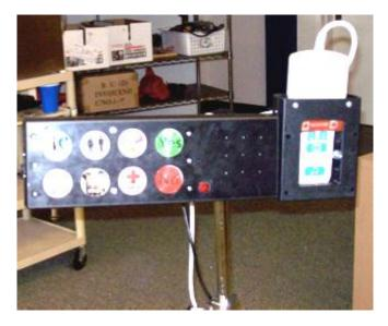
Fig. 9.1. The front view of the patient-nurse supplemental call system showing the large button display and hand-held call control caddy.
