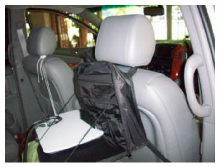
Fig. 9.11. The Video Window Viewer as installed in the client's family vehicle. The monitors are attached to the underside of the fold-down tray.
