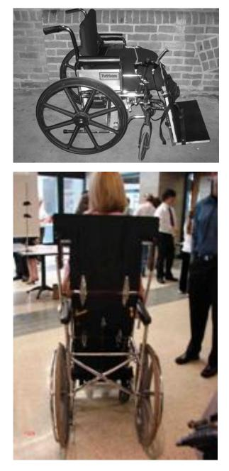
Fig. 9.12. The standing wheelchair. Top: wheelchair configuration. Bottom: standing configuration, rear view showing gas springs and 4-bar mechanism.
