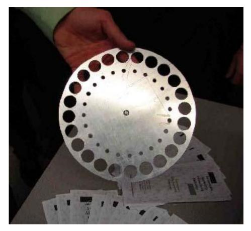
Fig. 9.9. Pill wheel showing 24 compartments and optical indexing holes.
